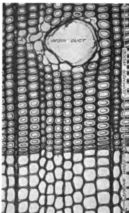
FIG. 327.—Transverse Section of Shortleaf Pine Showing Resin Duct. (Magnification 125 diameters.) (Bull. 101, U. S. For. Ser.)
